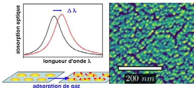
Fig.1. Shift of the plasmon resonance induced by the adsorption of molecules
